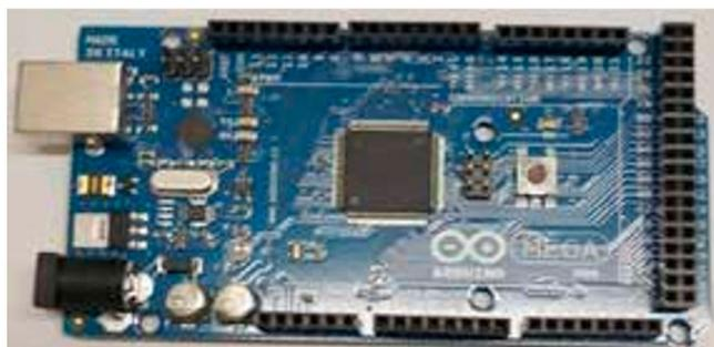
**Imagen 2.** Placa base Arduino MEGA 250 (Msc Yair Rivera, 2014)
